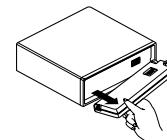
**3 Put the front panel into the protective case provided for safe keeping.**
