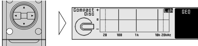
After the title screen, the display switches to the operation screen of the Equalizer Menu. Opening and closing the cover of the remote control (refer to page 4) switches between the open and closed states of the menu display and setting screen.
